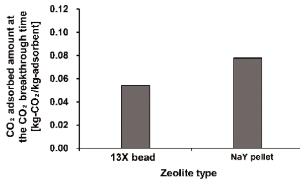
図4 Comparison of CO 2 adsorbed amounts between 13X bead and NaY pellet
